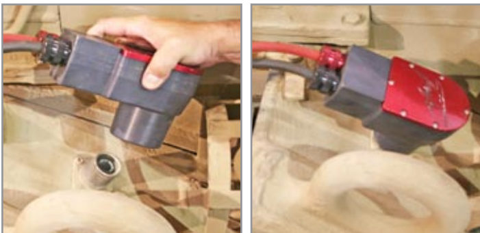
Figure 3.10.3 Attaching NATO DC Power Cable to vehicle
