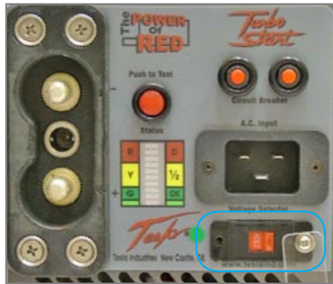
Figure 2.9.1 Input Voltage Selector Switch (outlined in blue)
