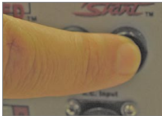
Figure 2.11.2 - Pressing Circuit Breaker
