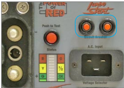
Figure 2.11.1 - AC Input Circuit Breakers (outlined in blue)
