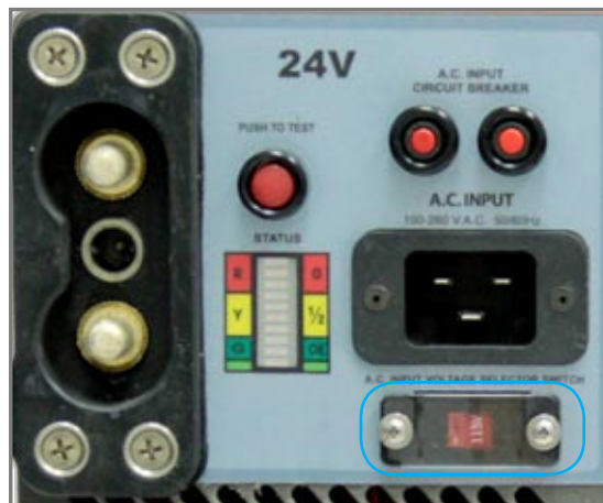
Figure 2.12.1 Input Voltage Selector Switch (outlined in blue)
