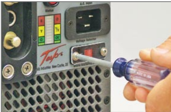
Figure 2.12.2 - Unscrew Protective Cover
