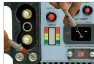
3.8.8 - Positive Probe to the Fastener Screw on the DC Receptacle.
