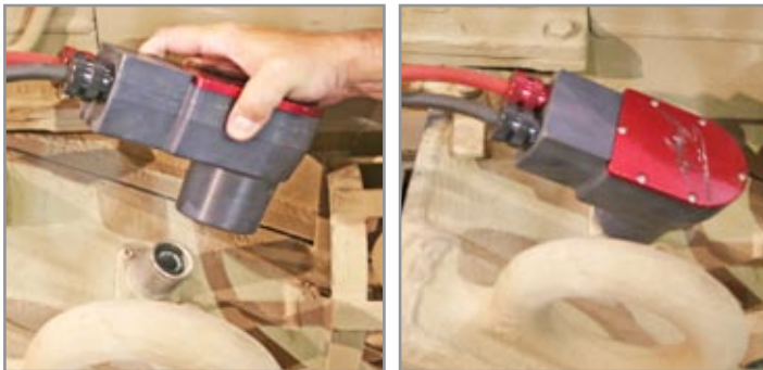
Figure 3.11.2 Attaching NATO DC Power Cable to vehicle
