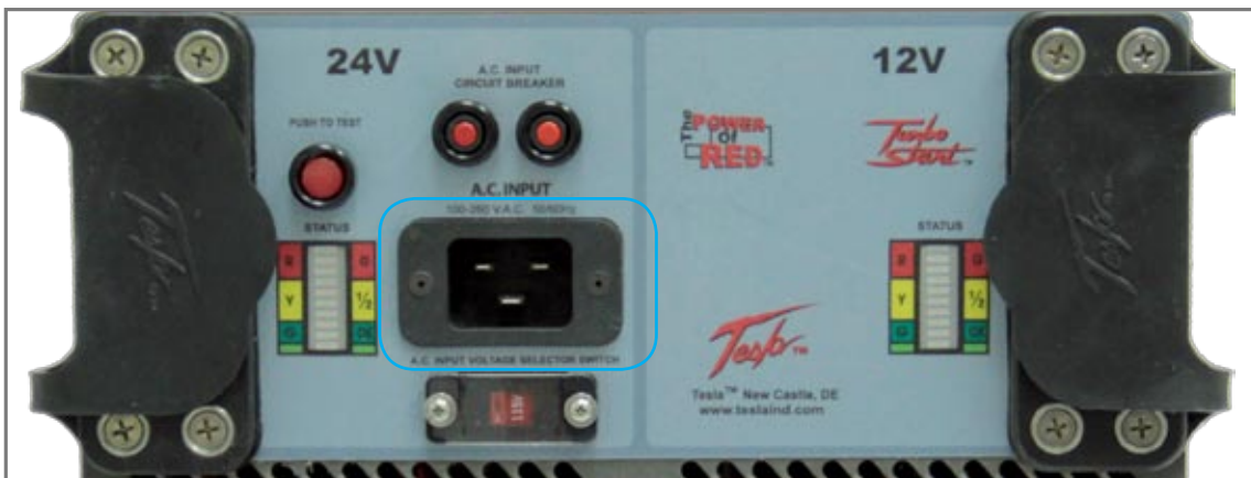
Figure 2.9.1 - AC Input Connector (outlined in blue)
