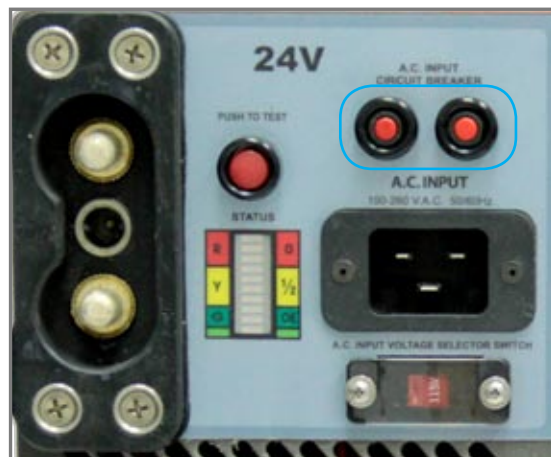
Figure 2.8.1 - AC Input Circuit Breaker (outlined in blue)
