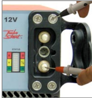
3.8.3 - DC Output Connector Positive Pin
