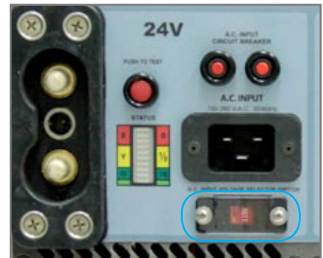
Figure 1.3.4 – TI3560 12-24 GPU Input Voltage Selector Switch
