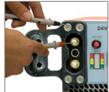
3.8.6 - DC Output Connector Negative Pin
