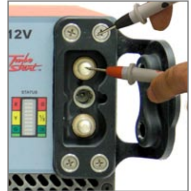
3.8.4 - DC Output Connector Negative Pin
