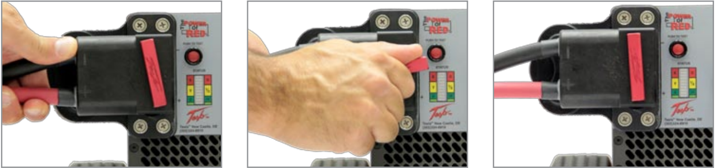
Figure 3.11.1 Attaching DC Power Cable to GPU
