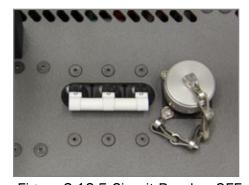
Figure 3.16.5 Circuit Breaker OFF
