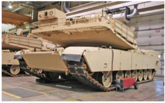
Figure 3.11.3 Starting vehicle with TI4200 GPU-24
