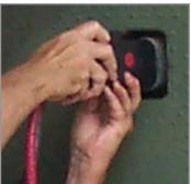
Figure 3.11.3 Attaching an Aviation DC Power Cable to aircraft
