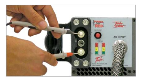
Figure 3.8.3 - Testing DC Receptacle
