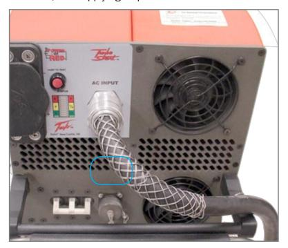
Figure 4.2.1 Circuit Breaker Selector Switch (outlined in blue)
