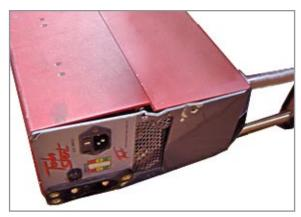
Figure 3.8.2 – Damaged Unit Misaligned Case with Bent Faceplate
