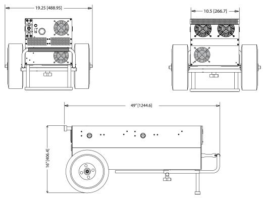
Figure 3.2.1 - TI4200 GPU-24 physical dimensions
