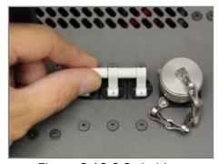
Figure 3.16.6 Switching Circuit Breaker ON
