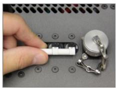
Figure 3.16.2 Switching Circuit Breaker OFF
