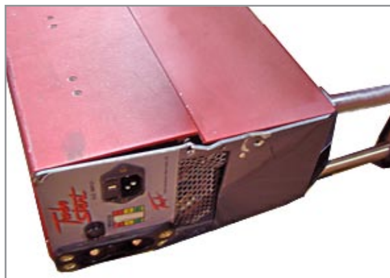
Figure 3.8.2 – Damaged Unit Misaligned Case with Bent Faceplate
