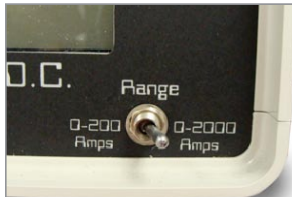
2.3.2 - Switched to 0-2000 Amps
