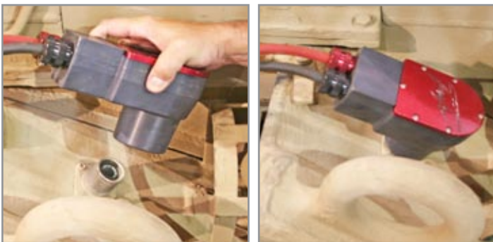
Figure 3.8.2 Attaching NATO DC Power Cable to vehicle
