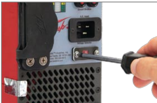
Figure 2.11.2 - Unscrew Protective Cover
