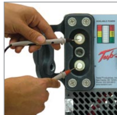
Figure 3.5.3 – Testing DC Receptacle
