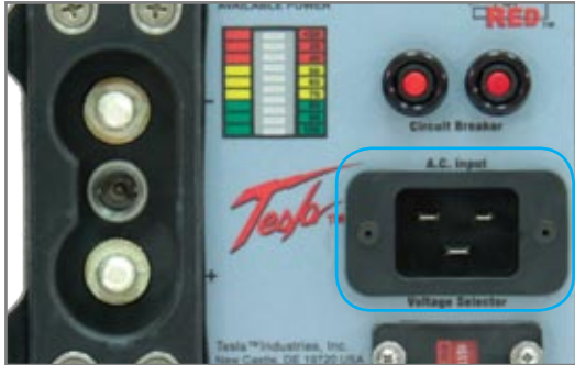
Figure 2.12.1 - AC Input Receptacle location (outlined in blue)
