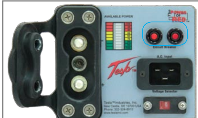
Figure 2.8.1 - AC Input Circuit Breaker (outlined in blue)
