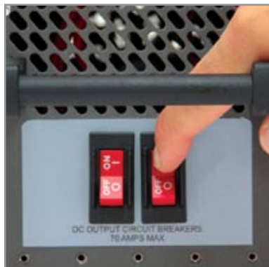
Figure 3.5.2 – DC Output Circuit Breakers has a 70 amps max
