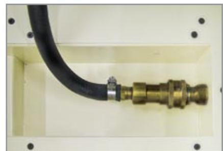
Figure 8.6.4 -Primary fuel line quick disconnect
