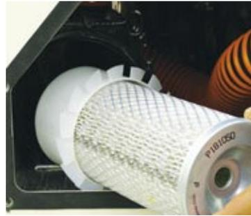
Figure 5.1.4 – Inspecting Air Filter
