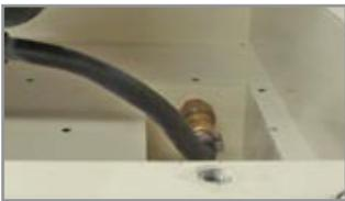
Figure 6.2.1– Supply Quick-Disconnect
