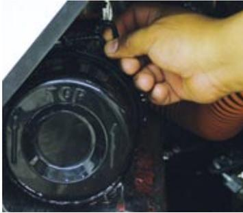
Figure 5.1.3 – Unscrewing Filter Cover
