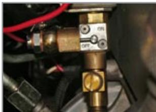
Figure 6.2.7– Manual Bypass “OFF” Position
