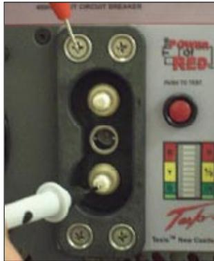
Figure 8.3.2 - DC Output Receptacle Positive pin
