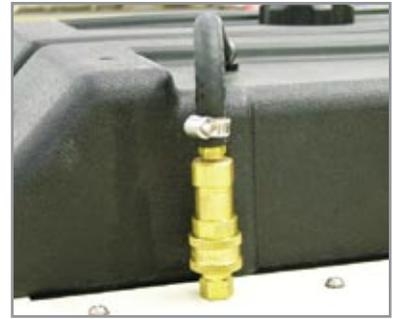
Figure 8.6.1 – Fuel return line quick disconnect
