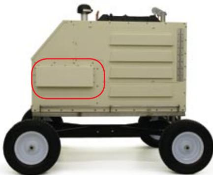
Figure 3.9.1 – GPU Exhaust Louver (outlined in red)
