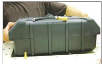
Figure 8.6.3 – Removing Fuel Tank
