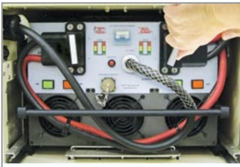
Figure 6.9.3 – Both DC Cables connected to GPU
