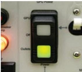
Figure 6.10.1 – Switch to AC Outlet Power
