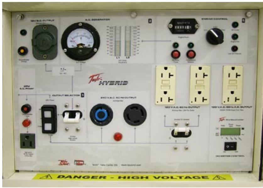
1 – 12 VDC Output-Indicator Light – Illuminates when 12 Vdc output is in use.
