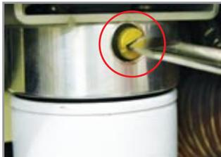
Figure 6.2.4– Fuel Filter Bleeder Screw
