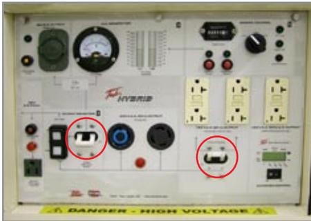
Figure 6.2.9– Location of Circuit Breakers
