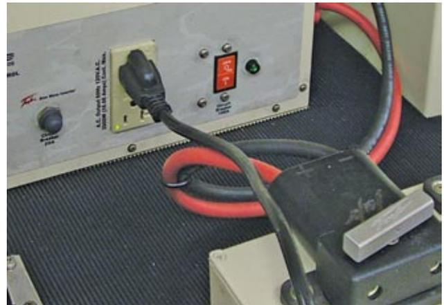
Figure 6.10.8 – Inverter GFCI Outlet.
