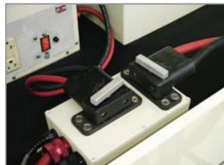
Figure 6.9.4 – Attach Aviation Cable DC connector to DC Junction Box
