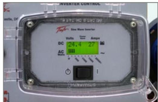
Figure 4.16.2 Inverter Display Panel
