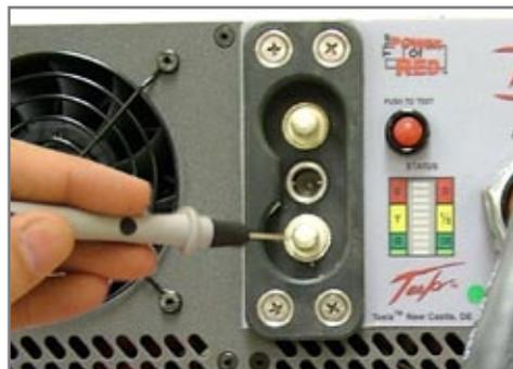
Figure 8.2.9 DC Output Receptacle - Positive Pin
