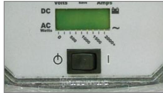
Figure 4.17.2 - Inverter On/Off Switch
