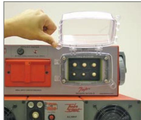
Figure 4.9.2 3-phase 400 Hz AC Input
