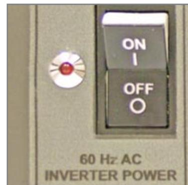
Figure 4.3.2 - 60 Hz Inverter Power Switch
