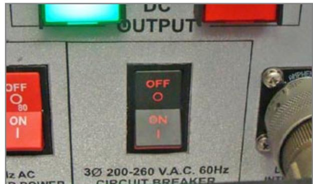
Figure 8.2.16 60Hz AC Input Circuit Breaker (set to “OFF” position)
