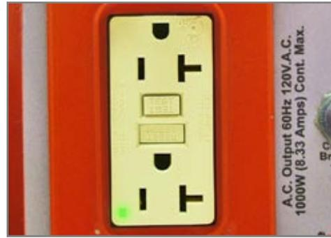
Figure 11.1.7 – 60Hz AC Power Outlet “ON” (green LED illuminated)
