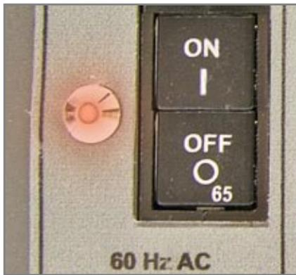
Figure 11.1.4 60Hz AC Inverter Power set to "ON" position (LED illuminated)
