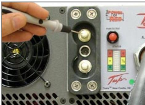
Figure 8.2.8 DC Output Receptacle - Negative Pin
