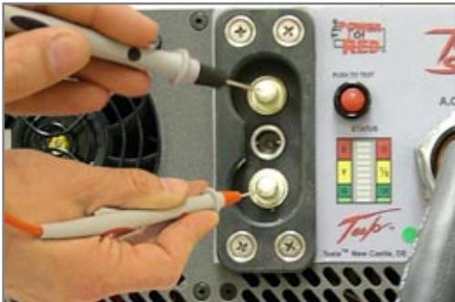
Figure 8.2.17 – Measuring voltage on DC Output Receptacle
