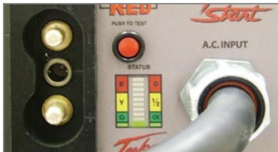
Figure 6.2.1 “Push to Test” and Status Meter
