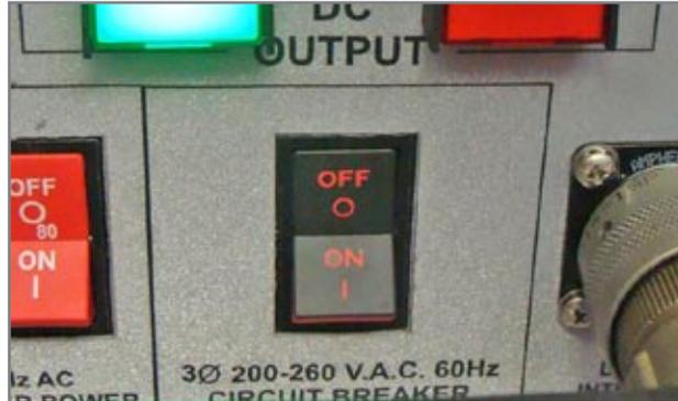
Figure 4.2.2 - 3-phase 60 Hz Input Circuit Breaker
