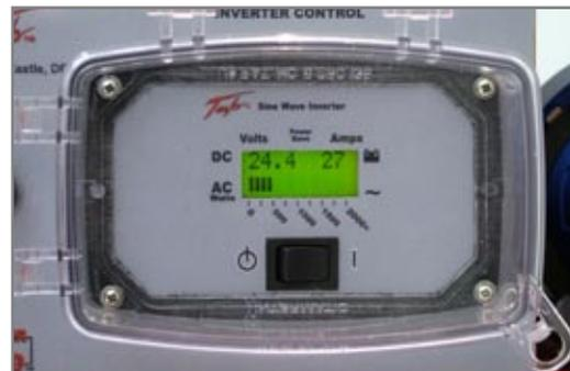
Figure 6.4.2 Inverter Display Panel with Switch set to “I” (ON) position.
