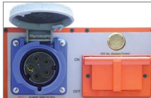
Figure 4.14.2 400Hz 200 Y 115 Output
