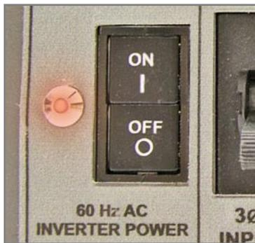
Figure 6.4.1 60Hz AC Inverter Power Switch “ON”
