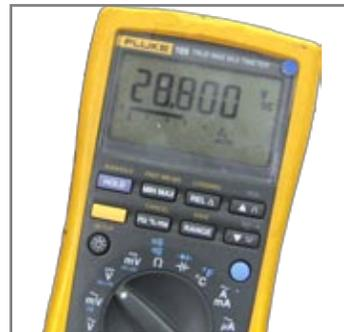
Figure 8.2.18 – Multimeter reading typical power cell voltage (with AC power)
