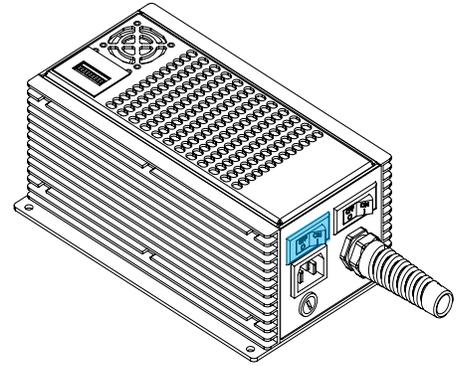
Figure 3.3.1 – AC Input Circuit Breaker
