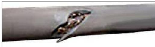
Figure 6.1.1 – Damaged cable
