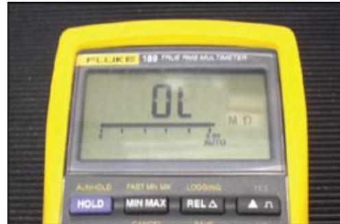
Figure 6.2.3 – Multimeter reading open circuit
