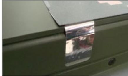
Figure 5.2.1 – Warranty Void stickers on the TI2000-308 3 kW Inverter System
