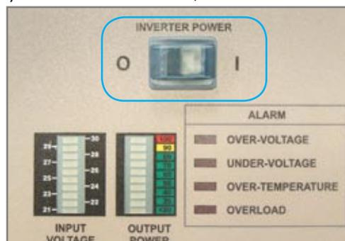
Figure 2.16.1 - Inverter Power Switch location (outlined in blue)
