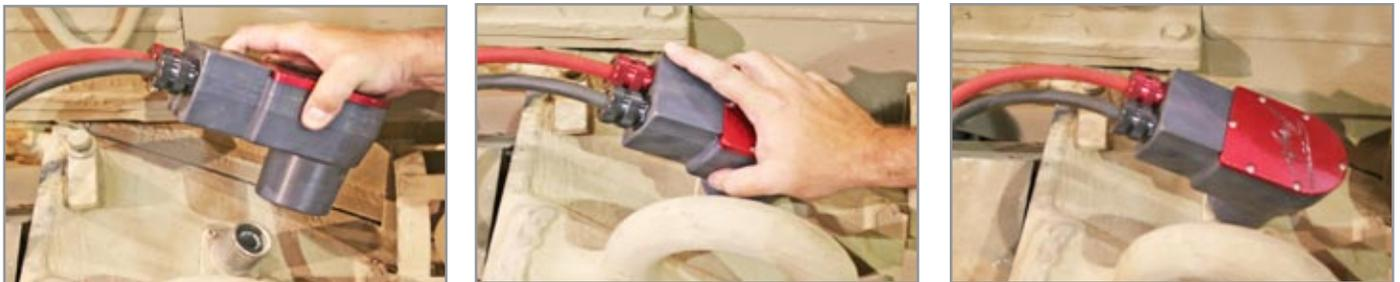
Figure 3.7.1 Attaching DC Power Cable to ground vehicle
