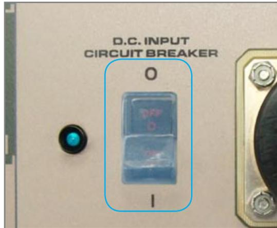
Figure 2.12.1 - DC Input Circuit Breaker (outlined in blue)
