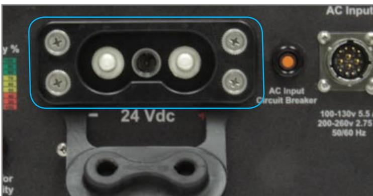
Figure 3.2.1 DC Output Connector
