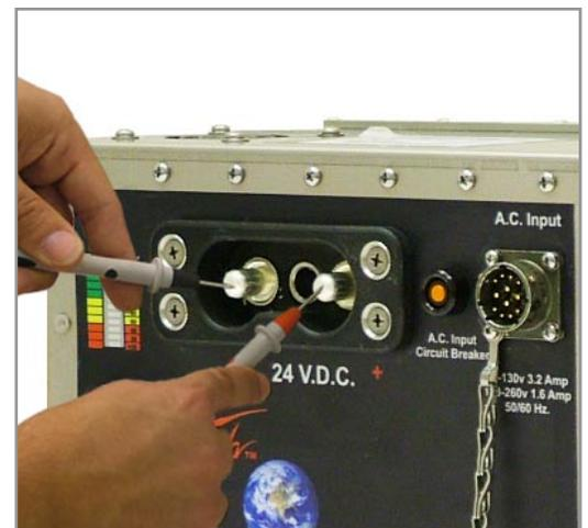
Figure 4.9.3 – Testing DC Receptacle
