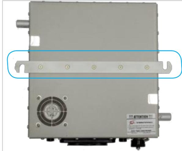
Figure 3.8.1 – Battery Lock-down (outlined in blue)
