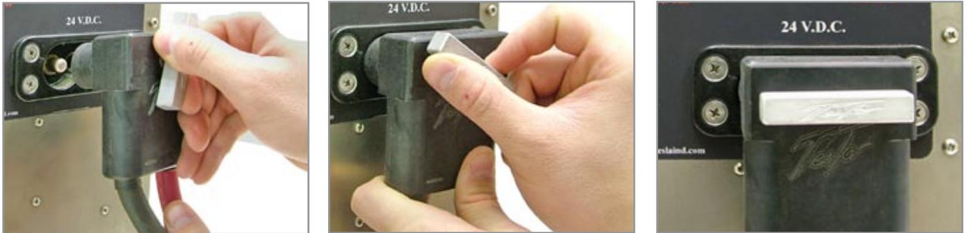
Figure 3.2.3 Attaching DC Power Cable to Unit
