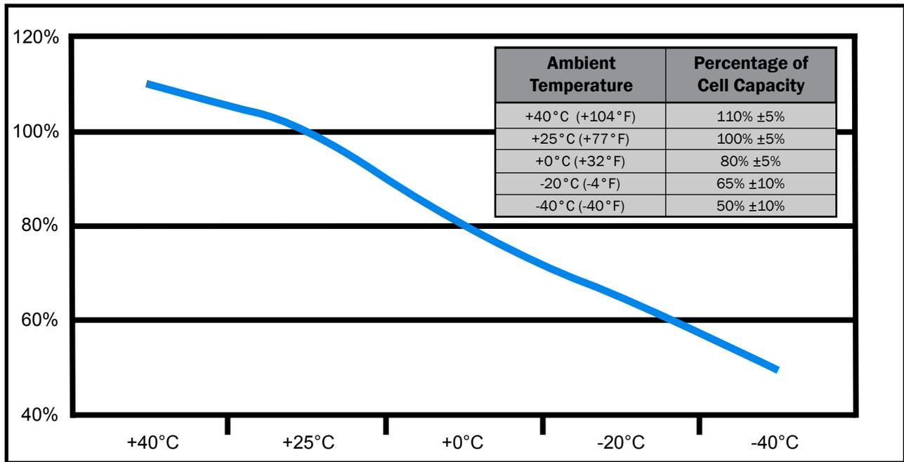
Figure 4.7.1 – Cell storage capacity versus ambient temperature
