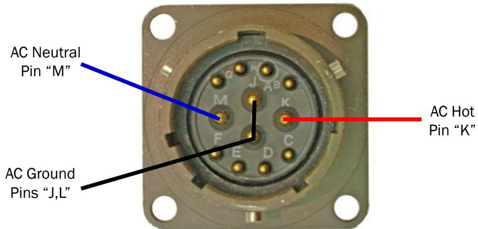
Figure 4.9.2 – AC Input Connector wiring diagram
