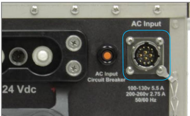
Figure 3.6.1 AC Input Connector (outlined in blue)
