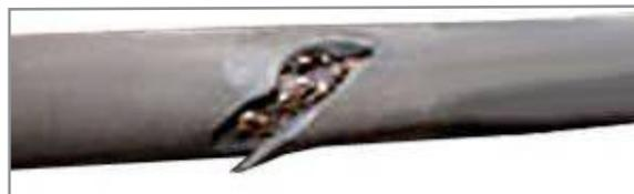
Figure 6.1.1 - Damaged Cable
