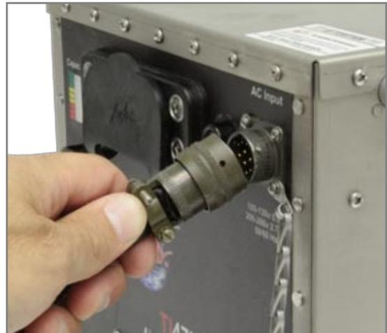
Figure 3.6.2 Attaching AC Line Cord
