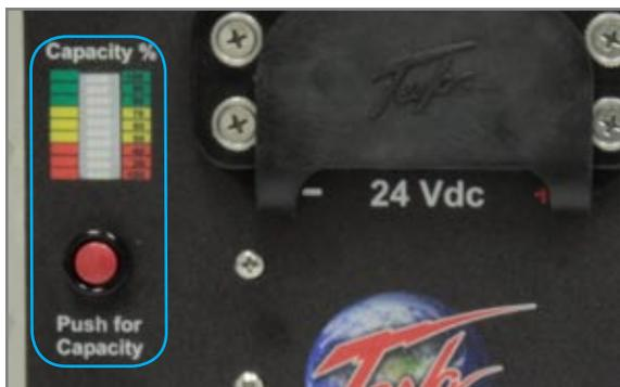
Figure 3.7.1 “Press for Capacity” button location (outlined in blue)
