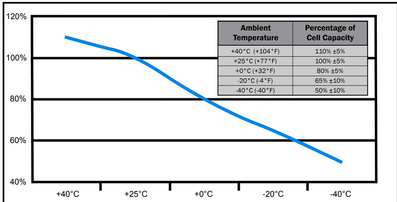
Figure 3.6.1 – Output power capability versus ambient temperature
