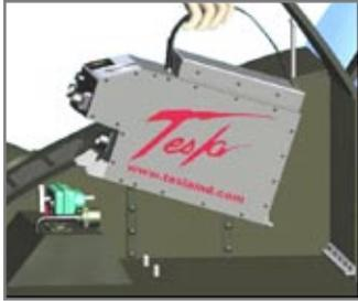
Figure 2.11.1 – Maneuver TI58D into battery compartment
