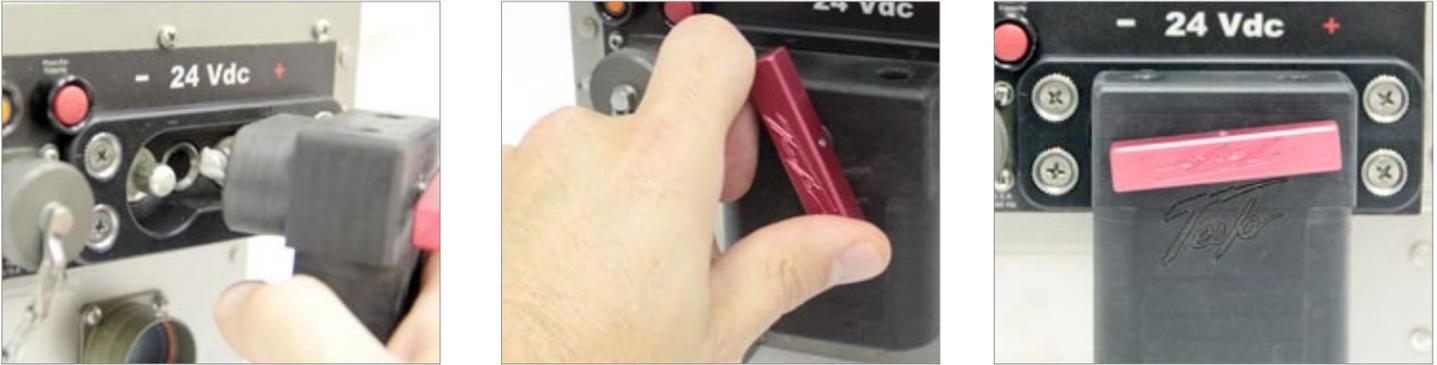
Figure 3.10.1 Attaching dc power cable to TI58D MPU-24
