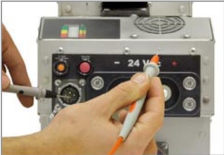
1. Place the negative probe on the ac ground probe ( J or L) and the positive probe on an exposed part of the metal case.
