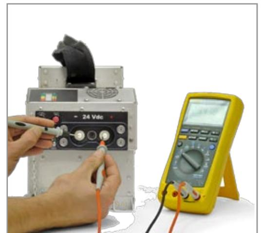
Figure 3.9.3 – Testing DC Receptacle
