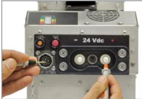
2. Move the positive probe to the dc positive post on the dc output connector.
