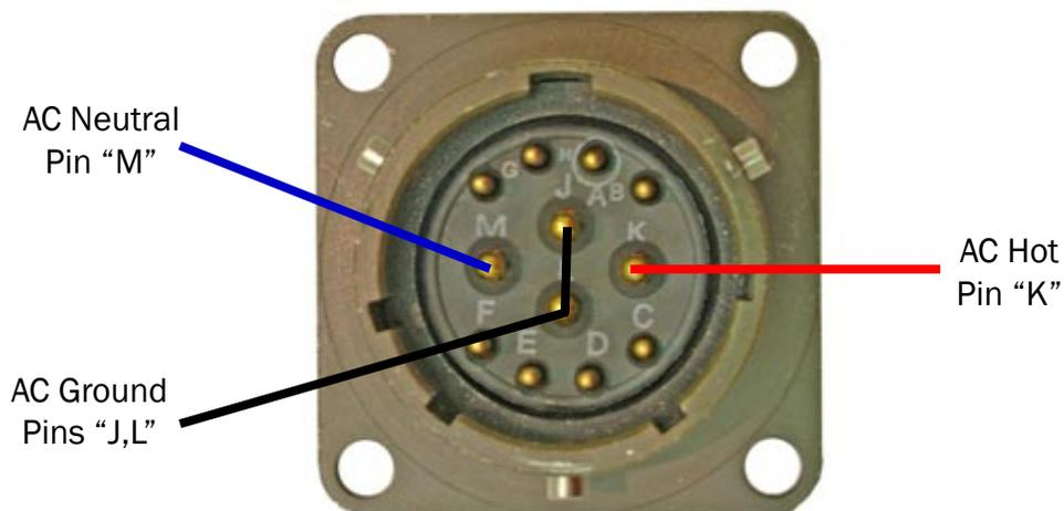
Figure 3.9.2 – AC Input Connector wiring diagram
