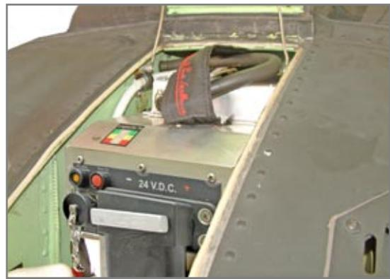
Figure 2.10.2 - Battery Compartment
