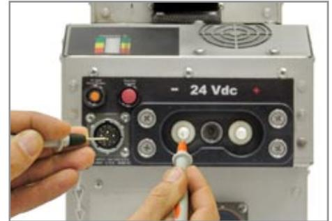
3. Move the positive probe to the dc negative post on the dc output connector.
