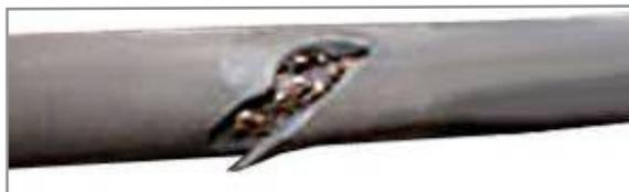
Figure 5.1.1 – Damaged cable
