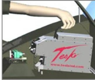
Figure 2.11.2 – Slide back flange into receiving lip
