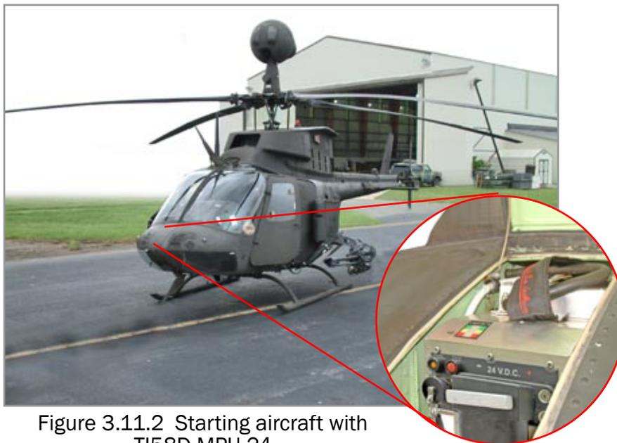
Figure 3.11.2 Starting aircraft with TI58D MPU-24
