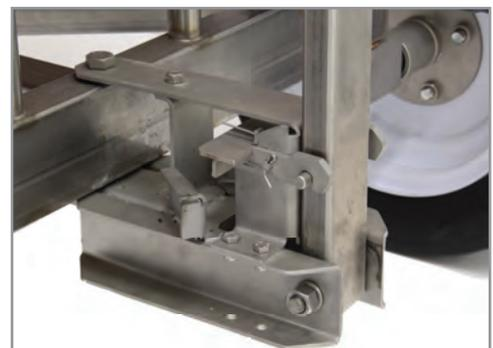
Figure 4: Tow Handle Release Pedal
