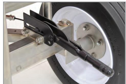
Figure 3: Hand Brake (activated)
