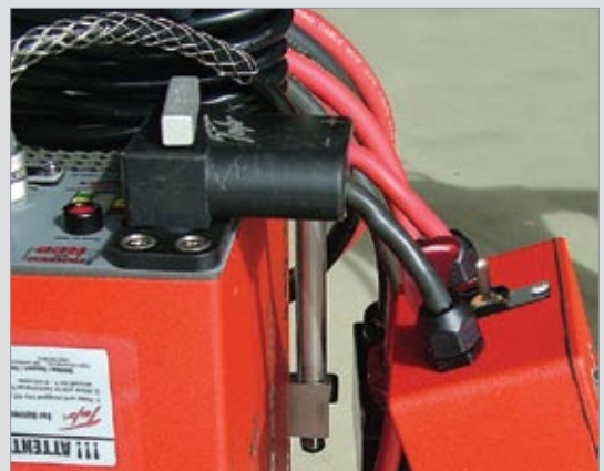
Figure 3: Rescue hoist control attached to a Tesla GPU.
