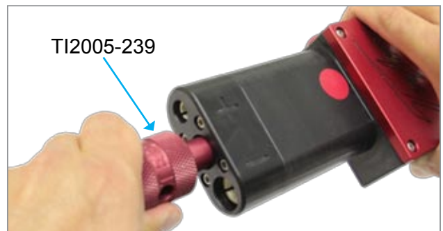
A - Insertion/Extraction Tool: TI2005-239 B - Positive/Negative Contacts: TI2005-251 C - Three Slotted Connector: TI2005-250
