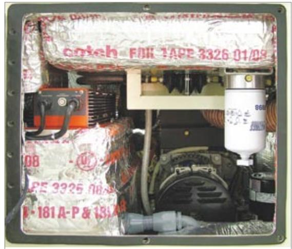
Left Engine Access Panel - Fuel Filter, Generator, Oil Cooler, and 2 internal Battery Chargers
