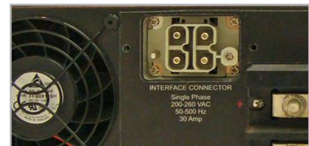
Figure 2: AC Input and Cooling Fan
