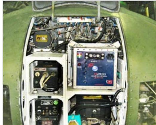
The TI47UH1 installed in helicopter.
