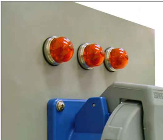
Figure 4.4.2 Indicator Lights OFF.
