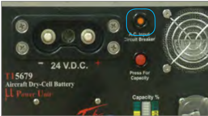
Figure 4.1.1 AC Input Circuit Breaker location (outlined in blue)
