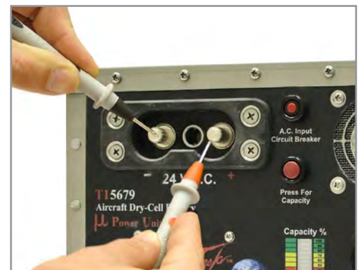
Figure 7.2.3 – Testing DC Receptacle
