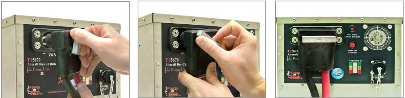
Figure 4.5.1 Attaching DC Power Cable to TI5679 MPU
