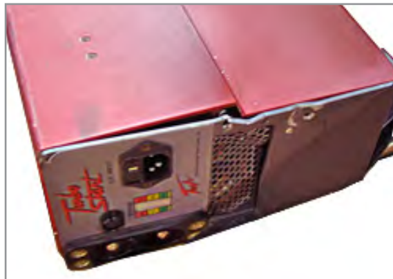
Figure 7.2.2 – Damaged Unit Misaligned Case with Bent Faceplate
