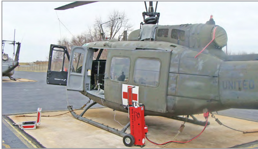
Figure 5.8.4 Starting UH-1 Huey Helicopter with TI3000 GPU-24
