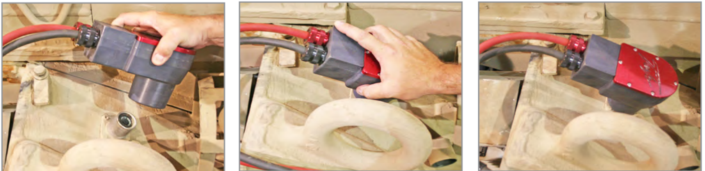
Figure 5.7.2 Attaching DC Power Cable to vehicle
