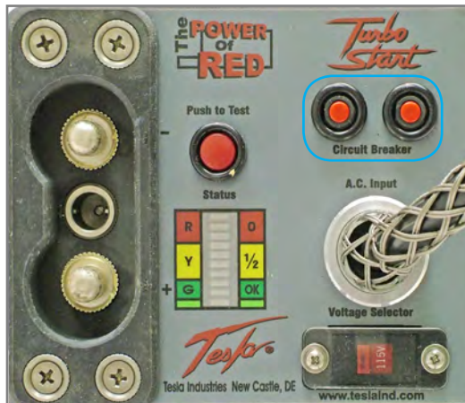
Figure 4.2.1 - AC Input Circuit Breakers (outlined in blue)
