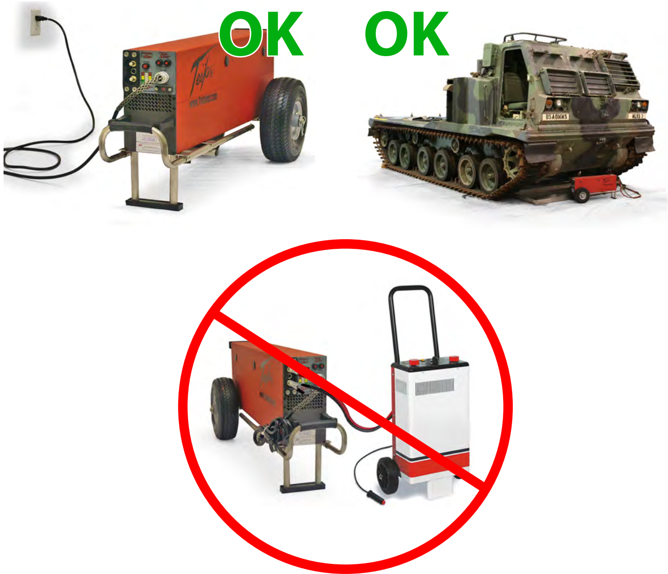
Figure 6.3.3 Proper and Improper Charging Methods
