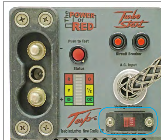
Figure 4.3.1 Input Voltage Selector Switch (outlined in blue)
