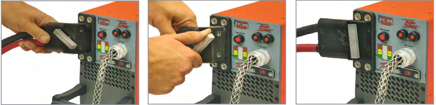
Figure 5.7.1 Attaching DC Power Cable to TIMV3000 GPU-24
